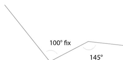
Seat and back can be adjusted with a fixed inclination angle.
